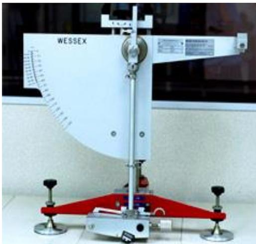
**The Pendulum Test is The Health & Safety Executive's (HSE) preferred method of testing, because it is portable and works in the conditions that slip accidents happen.**
