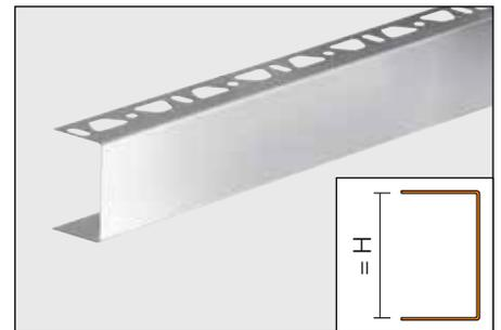
Schlüter®-KERDI-BOARD-ZA is a U shaped profile of brushed stainless steel with two perforated anchoring legs. It is suited for visible edges of partition walls and shelves.
